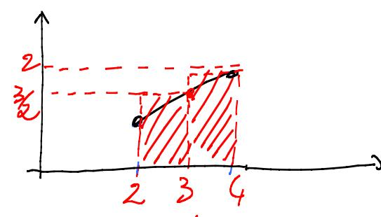
$$\begin{aligned}\text{S}(f, \mathcal{B}) &= \sum_{k=0}^1 (x_{k+1} - x_k) \sup f([x_k, x_{k+1}]) \\ &= (3-2) \sup f([2, 3]) + (4-3) \sup f([3, 4]) \\ &= 1 \cdot \frac{3}{2} + 1 \cdot 2 \\ &= \frac{7}{2}\end{aligned}$$
